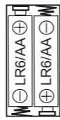
Remote control The remote control operates with 2 x 1.5V AA/LR6 batteries (not included)
