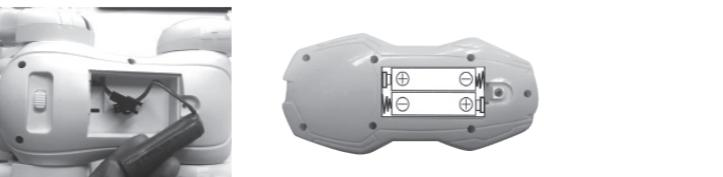
The robot operates with 1 x DC 3.7V 500mAh (included)
